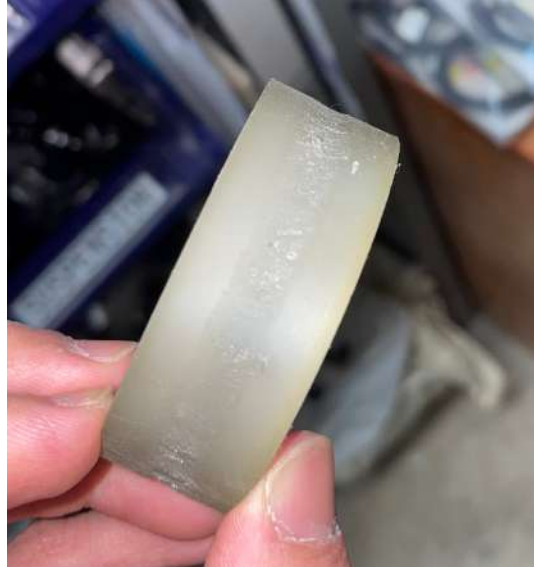
Figure 3.6d: Damaged Flywheel Rubber
