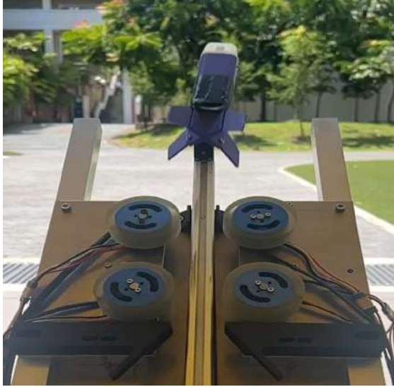
Figure 3.6e: Inaccurate Launch due to inconsistent Flywheels Angular Speed
