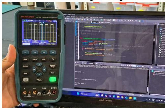
Figure 4.1.3f: Oscilloscope showing PWM signal of 500.1 Hz, in an attempt to move it by 100 steps with a PWM frequency of 500 Hz. (Motor driver settings: 400 steps per revolution.)
